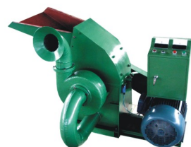
TFS420 (粉碎机 hammer mill without cyclone)
